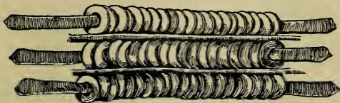
Fig. 44. SUGGESTED CONSTRUCTION OF BANDED MAIL
