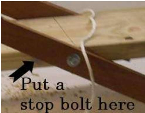
This picture shows the stop bolt in place. These are the two left over 1 inch screws you had after screwing down the wheels.
