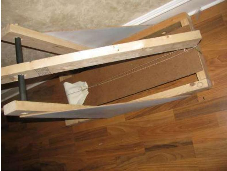
With the trebuchet in the loaded and ready to fire position as shown in the picture below you put the little ring you made onto the straight nail. When the catapult fires this little ring will come off the nail and allow the pouch to open and release the tennis ball.
