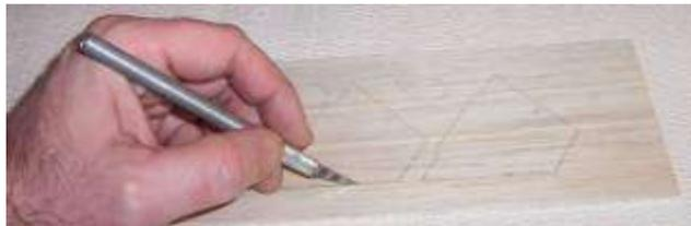
The above illustration shows the fins for the balsa wood rocket. They are stamped and pre-cut but you will need a sharp knife to cut the small tabs and remove them from the sheet of wood.
