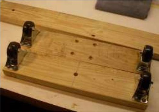
Optionally, you can attach the wheels to the 24 inch boards before you attach the boards to the main board. You can see here I have everything pre-drilled and ready to assemble.
