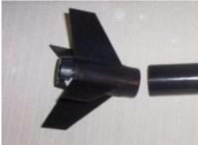
The fins and engine mount are glued together and ready to put mount to the rocket tube.
