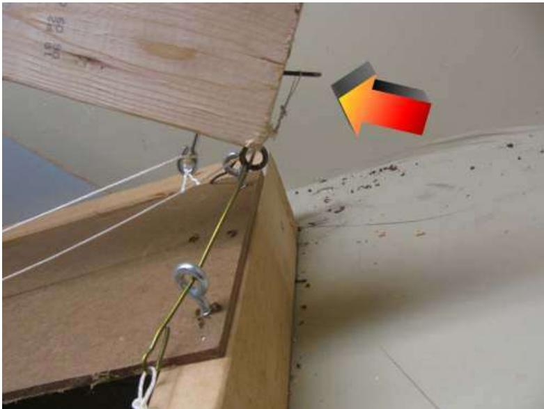
The Locking mechanism and trigger.- The coat hanger goes through one eyehook then through the eyehook on the swing arm and finally through the eyehook on the far side. Pulling on the string releases the swing arm.
