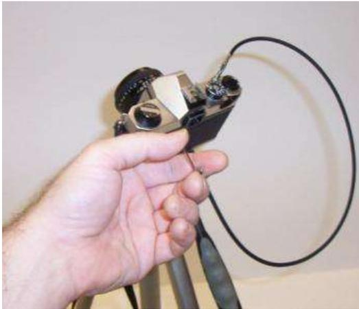
A Shutter release cable is an inexpensive little cable that will allow you to hold the shutter open for long periods of time without touching the camera. This cable has a little lock on it so I can open the shutter and then lock it open.
