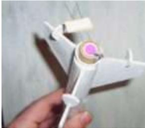
Now you install the engine into the rocket then place the rocket onto the launching pad by threading it onto the guide bar.
