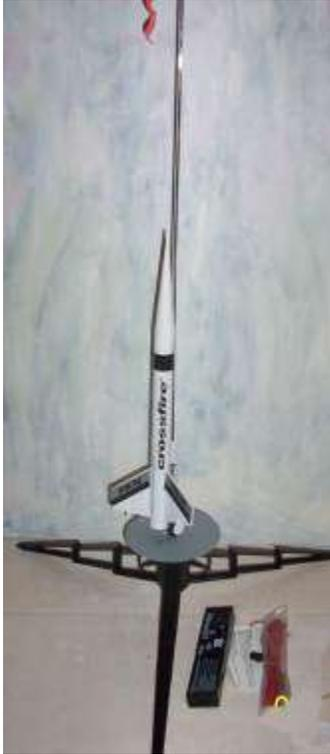
Here is a typical launching pad. This is the one that comes with the Estes tandem-x kit. It is about three feet in height and how you see it in this picture is similar to how you would use it to launch rockets. The rocket sits on the metal plate and when it is launched it runs up the metal rod. There is a small guide tube on the rocket that the rod goes through.
