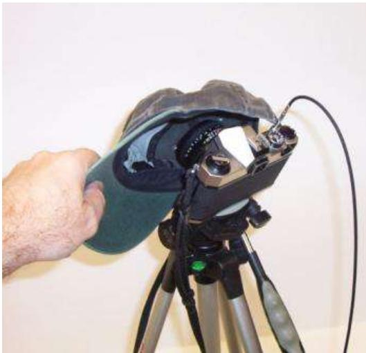
Here is the best way to take your pictures without introducing any shake. Cover the lens with a dark object like a hat, trip the shutter release so the shutter is open, then remove the hat for your duration of exposure. After your time is up put the hat back over the lens and then close the shutter.
