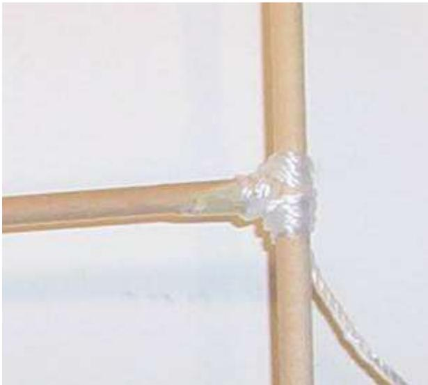
The best technique for assembly is to put the two pieces together where you want them connected then apply a piece of masking tape to hold them in place. Then you wrap the joint with your string. Finally you cover the string with masking tape. This makes a really strong yet lightweight joint.
