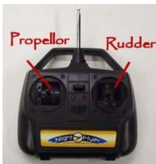
Here is the transmitter for the plane above. The joystick on the left is one channel and it controls the propellor. The joystick on the right is on a second channel and it controls the rudder which turns the plane. This is a simple two frequency set up and something you can expect in a very basic and inexpensive beginner plane.
