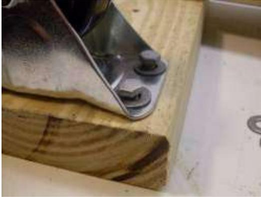
Now turn the Kart over and bolt down the wheels using the 1/4 inch by 1 inch screws. put a washer under each one. The picture shows a nice assembly tip. Do not put a screw in and tighten it. It makes it hard to get the other ones in. Put all four in and wind them down partially. Once the wheel is lined up nice and straight then tighten all four down.
