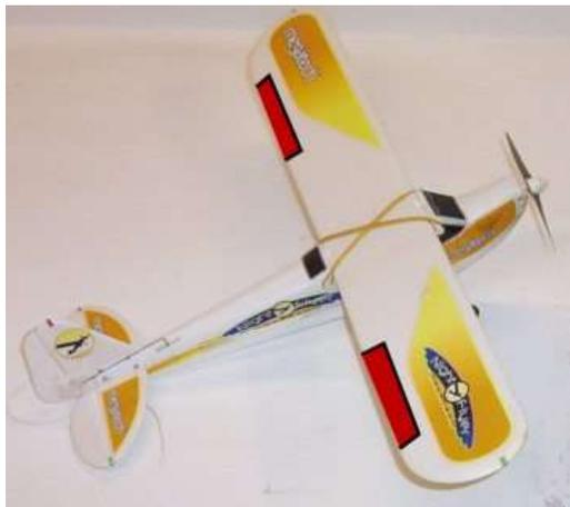
This picture shows an airplane with the Ailerons in red. When the aileron signal is activated the aileron on one wing tilts down while the aileron on the other wing tilts up. This is an effective way of rolling the airplane roll one way or the other.
