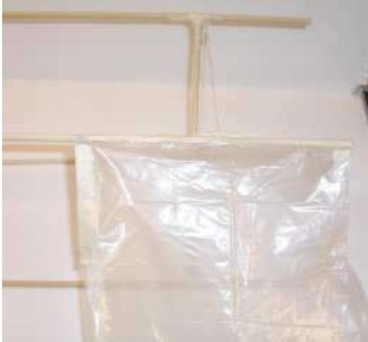
Using masking tape attach one end of the plastic to one of the bars as shown.
