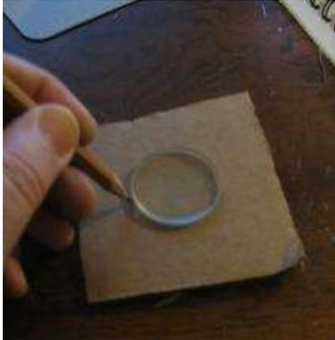
Put a lens down on the square of corrugated cardboard and draw a line around it. Do this whole process for both lenses. (make two of these)
