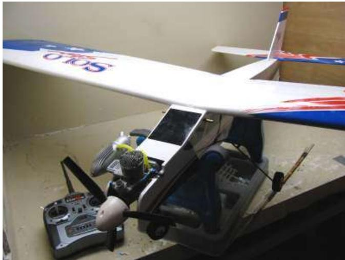
This is one of those airplanes. It is made out of balsa wood that is covered over by a special skin. This is a large plane that is about 4 feet long with a 5 foot wingspan. This type of plane is called an "ARF" which means almost ready to fly. All of the hard work has been done and about 10% of the work still remains for you to do. But this still could amount to a good 20 hours of work. It did for me. I built this very plane.
