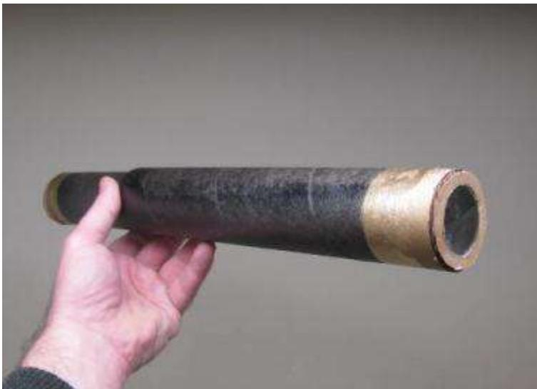
Slide the thinner tube into the thicker tube and your telescope is complete. Have fun!
