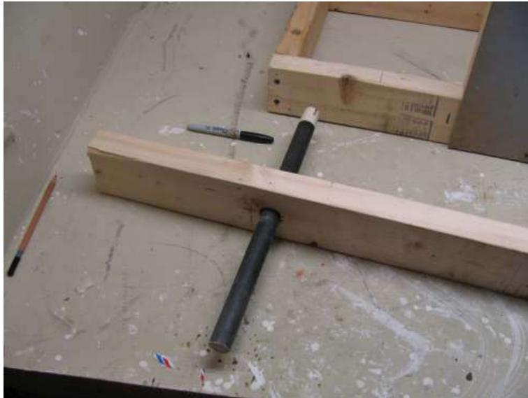
Now this is a little bit tricky but you have to put two eyehooks and 1 nail on the other end of the swing arm. Do it as shown in the picture. The nail is a straight nail with the head cut off. This is important, you don't want any kind of head on the end of this nail so the string and loop can easily slip off it. When the string and loop slips off this nail the pouch is opened and the projectile flies.
