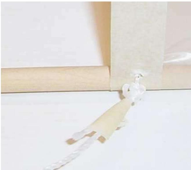
Attaching the string to the kite can be a little tricky but it will be strong enough if you cut a small hole in the masking tape and then wrap the string right around the wooden stick.
