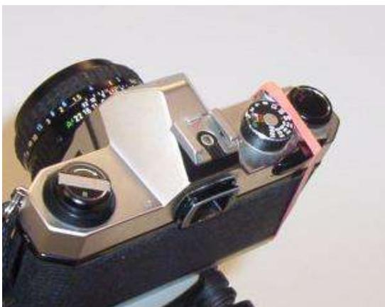
Alternatively, you don't need a shutter release cable. You can use a rubber band just like I have shown here. I have used this method very successfully. Just make sure you do it in conjunction with the hat method of exposing the film.
