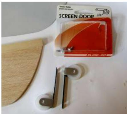
This project uses a variety of easy to find materials but the one important thing you are going to need is a pair of pulleys. It is important to have these so you can get a real easy and smooth riding up the string to the kite. I picked up a pair of screen door pulleys at the local hardware store.
