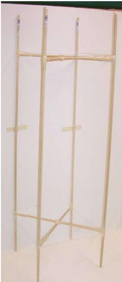
This picture shows the completed frame. Note that I have taped two of the uprights right up against a wall. This made it a lot easier to work with. If you are working alone you might want to use this technique. It is really handy.
