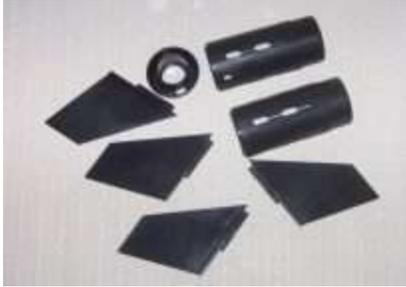
The Plastic Model Rocket is much easier to build and this picture shows the engine mount and the fins.
