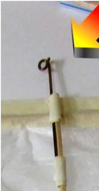
At the top of the vertical mast tape a paper clip that has been formed with a loop at the end of it. Be sure the loop extends past the top of the vertical mast.
