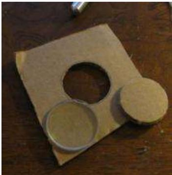
Using an X-acto or razor knife cut the circle out. You can use scissors but it is rather difficult because you will tend to bend and distort the cardboard. Try to cut the circle so the hole is just a tiny bit smaller than the lens. Maybe about  $1/32$  of an inch
