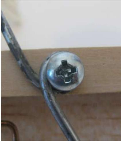
This second wire is about eight inches long. Bend it so it has a loop right in the middle that your screw can fit through. This will act as a pivot. When you do secure this to the boat you will only insert the screw far enough to hold tight but it needs to allow the wire to pivot freely. The head of the screw acts as a plate to just hold the wire on.
