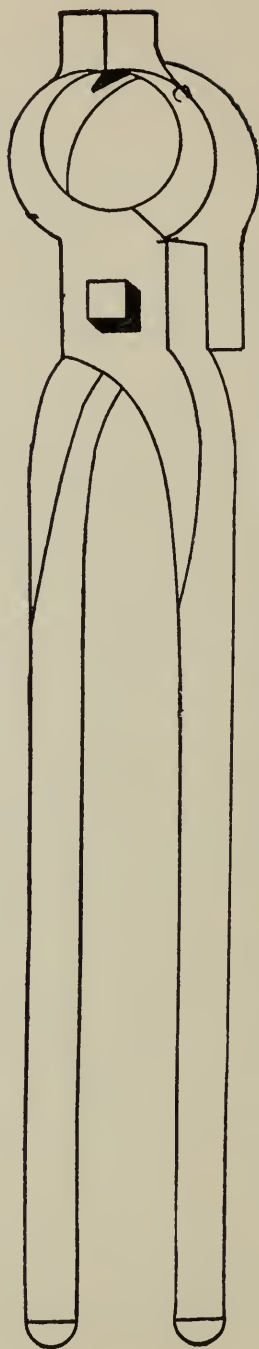
Fig. 5. Tongs specially made for dressing old chisels and all similar tools.
