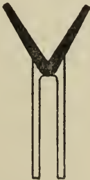
Showing piece split and forged to shape of jaw.
