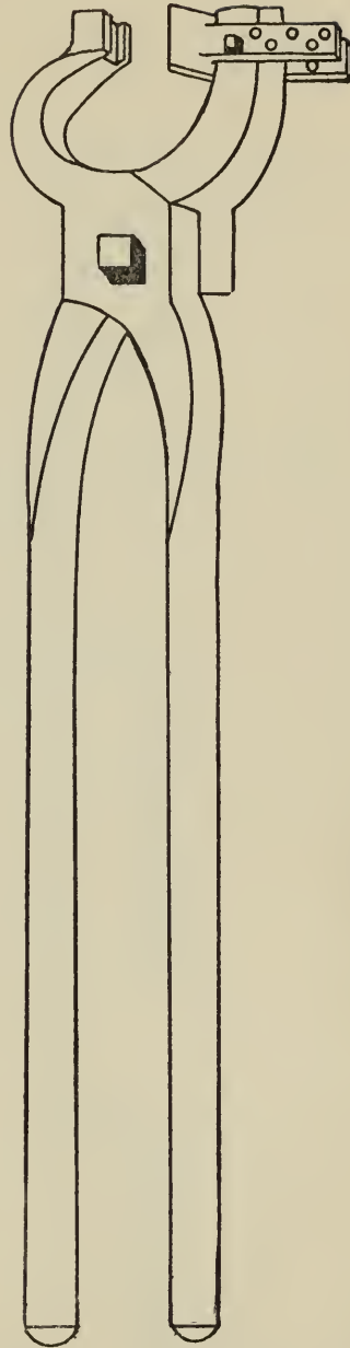
Fig. 4. Adjustable tongs regulated for holding largest size.
