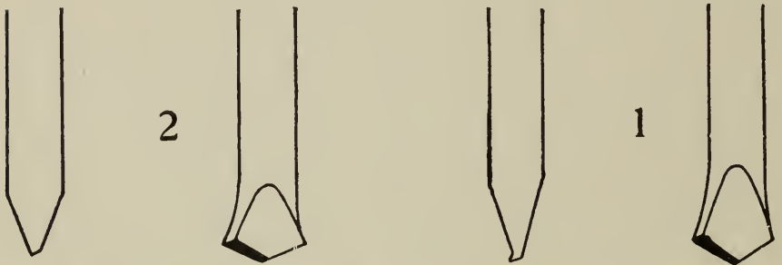
Fig. 23. Illustrating front and side views of flat drills, for hard and soft material.
