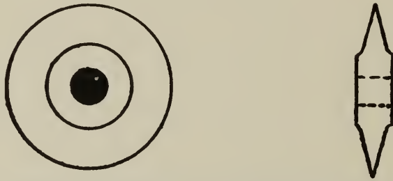
Fig. 110. Flat and end views of circular blade for pipe cutter.
