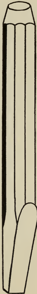
Fig. 57. The calking tool.
