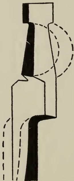
Illustrating how jaws are forged and bent to shape.
