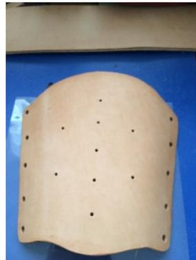
At this point you can apply leather dye or acrylic paint. Then after 24 hours put a leather finish on it such as Eco-Flo super shene (Tandy product) until it dries thoroughly another further coat may be applied but after this too is completely dry. Buff to a shine with a lint free cloth.
