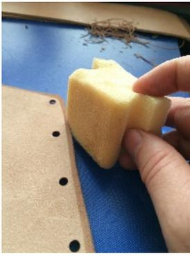
Wetting the edge of leather prior to using a slicker helps to burnish the material and neaten the edge.
