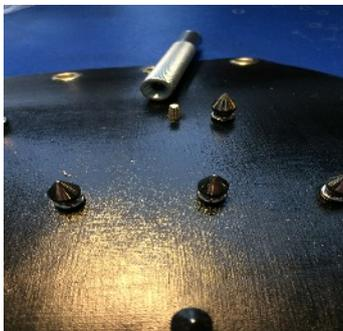
We can now fit the spike rivets to the main gauntlet body. There is a special punch that accommodates the spiked portion. There are two types of spike rivets one which is a long point and the pictured which is a shorter version.
